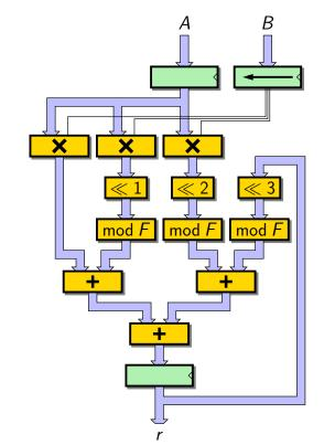
• feedback loop for accumulation of the result
